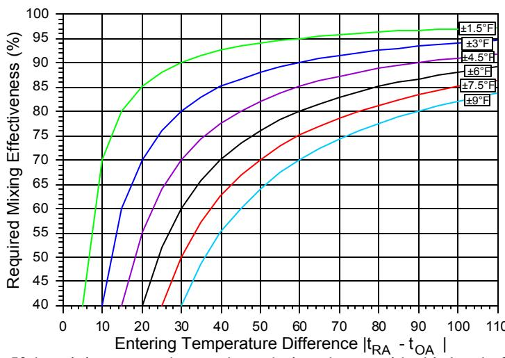
If the mixing system has not been designed to provide this level of mixing, the error in the mixed air temperature sensor can result in excess energy usage. This excess energy will either be the result of the sensor calling for too much mechanical cooling or it will be the result of the occupants turning down the thermostats because they are too hot.
